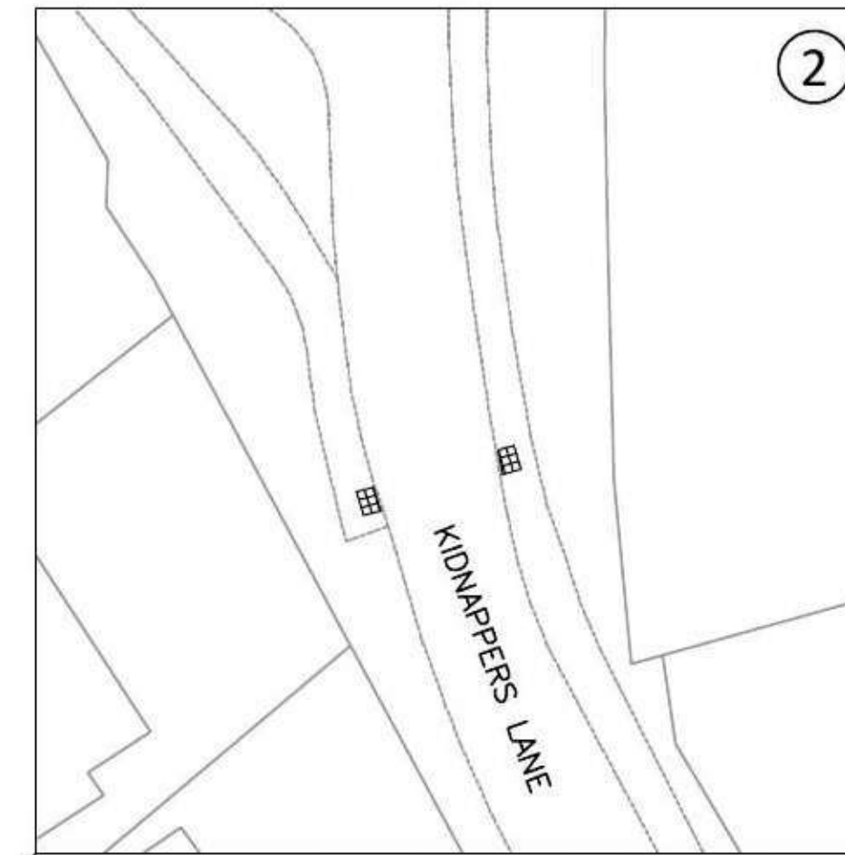
Kidnappers Lane pedestrian crossing, proposed dropped kerbs, pram ramp and tactile paving.
